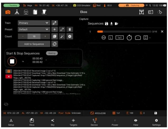
Pressing on the Logs button toggle the Logs from Capture module. All recent logs are displayed.
