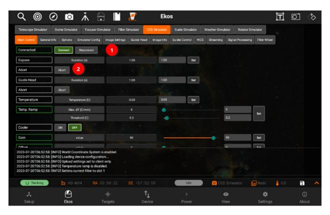
Some buttons show the active button (1), and a different button can be set active simply by pressing it. Other buttons (2) only send the action once pressed and we can tell if it was successful from the property status (3).
