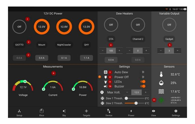
Power tab provides access to StellarMate Pro power dashboard and environmental sensor measurements. The top half of the dashboard controls the DC, PWM, and variable voltage outputs, while the bottom half includes measurements, settings, and sensor widgets.
