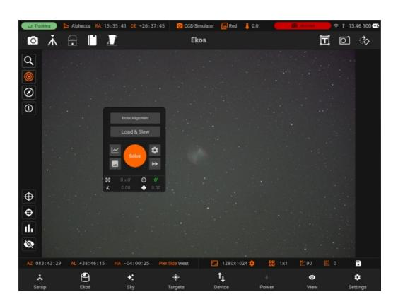
The Align module enables highly accurate GOTOs and dead-center target images by utilizing plate-solving. The process starts with capturing an image and plate-solving it to get the exact sky coordinates. Once the coordinates are obtained, the mount is synchronized and then commanded to slew to the correct target position. This cycle repeats until the mount is within a few arcsecs from the target.
