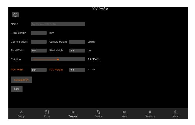
After setting the Focal Length, Camera width & height and pixel width & height, the FOV can be calculated by pressing the Calculate FOV button.
