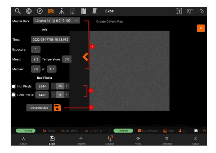
After creating a master dark, you can create a defect map for your camera. Usually, defect maps are used when dark frame subtraction does
