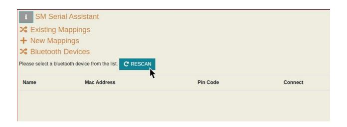
9. If you find your device, enter the pin code and then click on the Connect button. (eg. Shoestring Astronomy HC-06's pin code is 1234, you can find the pin code number by finding the bluetooth device's documentation made by the manufacturer)
