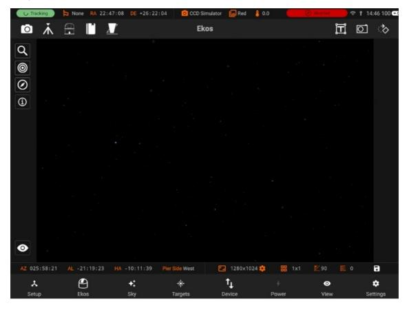
You can center the mount to a specific target in the main image if plate-solving was successful. From Ekos Align module, Capture and Solve an image. If successful, an orange align icon is displayed in the Main Image View indicating that solving is successful. For any subsequent images captured and displayed in the Main Image View, you may now select the target by tapping on it. A red bullseye animation designates the target.
