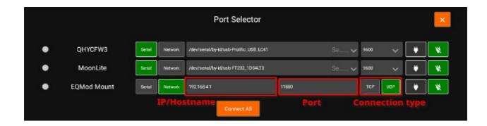
For network devices, you have to specify the host-name or IP of the device and the port. Also you can choose the network type (TCP/UDP).
