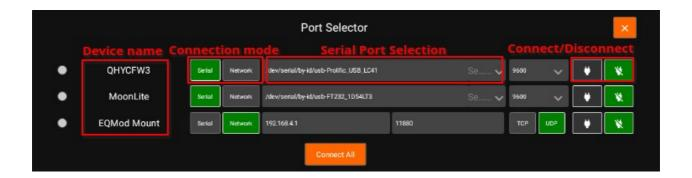
When connecting a serial device, you can specify the port by selecting from the drop-down or typing it in the text field
